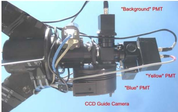
Fig. 2- Triple Photometer at prime focus
