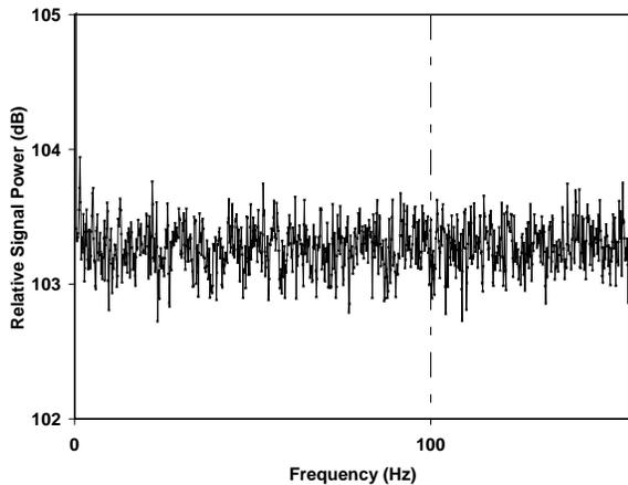
Fig. 12 Power spectrum of weak 100 Hz signal ( $RSA=1/5000$ )
