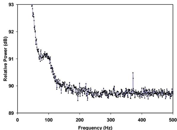
Fig. 15--A 371Hz “signal” in spectrum of HD195034 plotted in Fig. 14. The increase in background power at low frequencies is due to atmospheric scintillation
