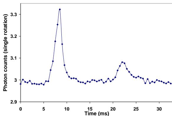
Fig. 5—Average light curve for 71,000 rotations of the Crab pulsar (B channel) during a 40min observation
