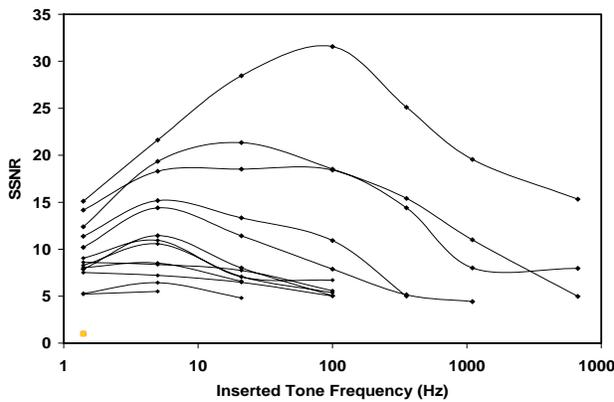
Fig. 8 Variation of SSNR vs frequency for curves of constant RSA
