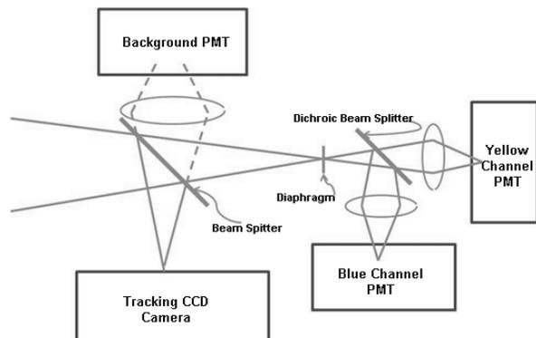
Fig. 1—Schematic of Triple Photometer. Note that the diaphragm is reflective to improve detection of background light
